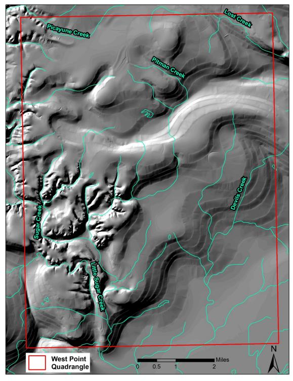
Figure 1: Raster image of the bedrock surface of the West Point 7.5' Quadrangle using a "hillshade" effect. Image generated from the bedrock topography lines drawn at 25-foot contour intervals.
