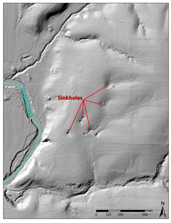
Figure 3: LiDAR image with "hillshade" effect to illustrate karst geology in the northwestern part of the West Point Quadrangle. Multiple sinkholes were identified in the Soil Survey of Lee County (Lockridge, 1979), however these were not able to be verified during field reconnaissance.
