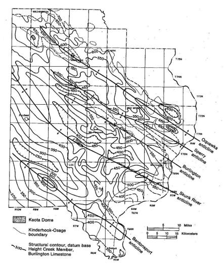
Figure 2: Structural contour map of southeast lowa. Contours are drawn on the base of the Haight Creek Member of the Burlington Formation (Osagean Series). A number of anticlines are shown and are flanked by synclines (unlabeled). (From Harris and Parker, 1964, plate 2)
